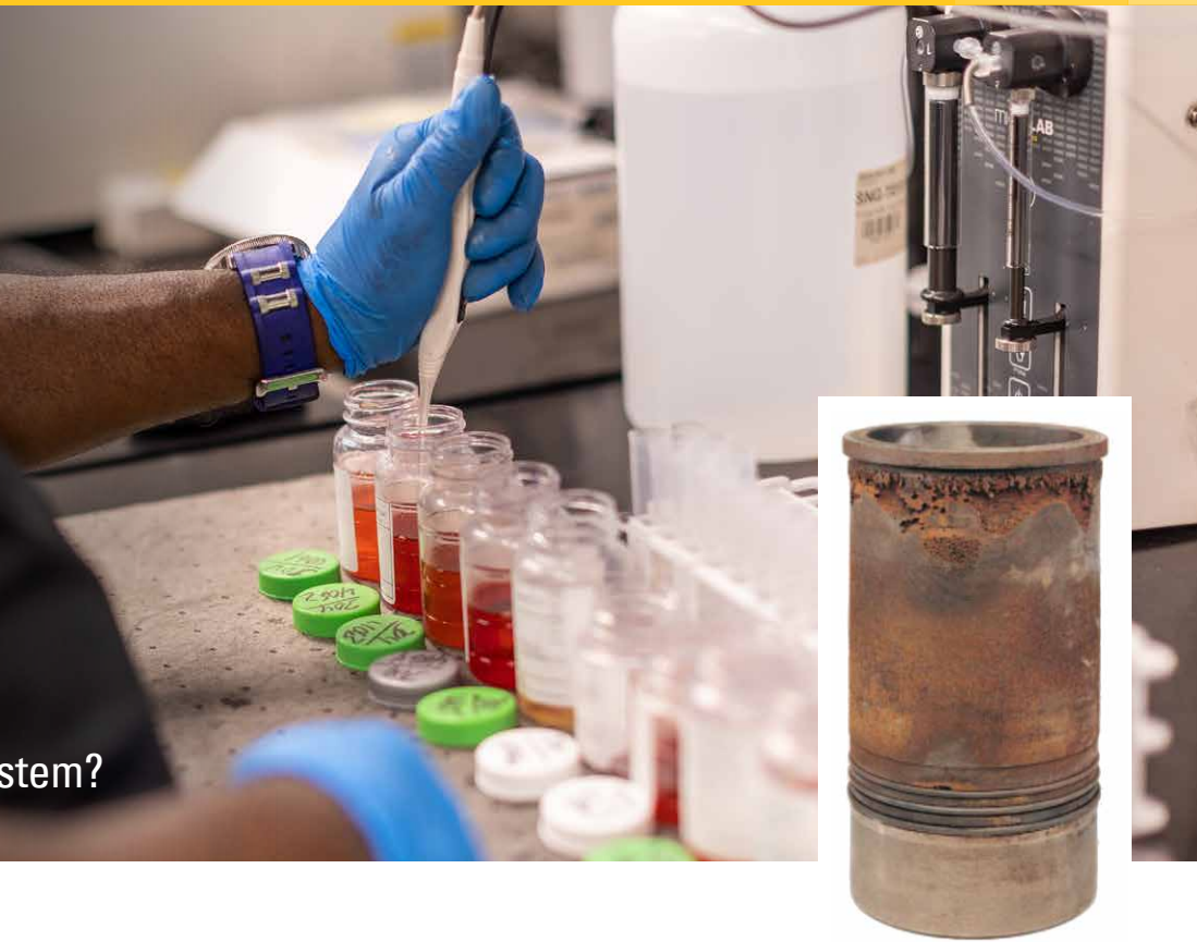
Corroded cylinder liner, resulting from neglected cooling system
