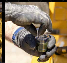
Secure cap onto sample bottle
