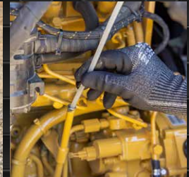
Insert tubing into the fluid sump
