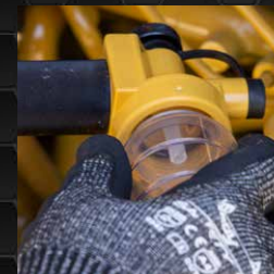
Insert tubing 1" into head of the vacuum pump
