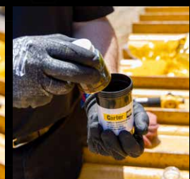
Place sample into the shipping cylinder
