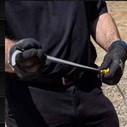
Measure tubing to length of dipstick
