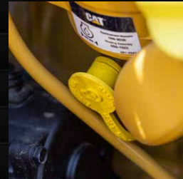
Dust cap on valve
