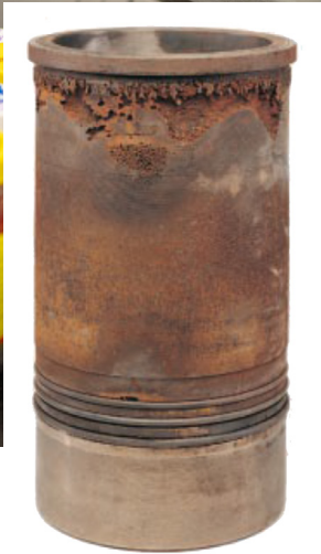
Corroded cylinder liner, resulting from neglected cooling system
