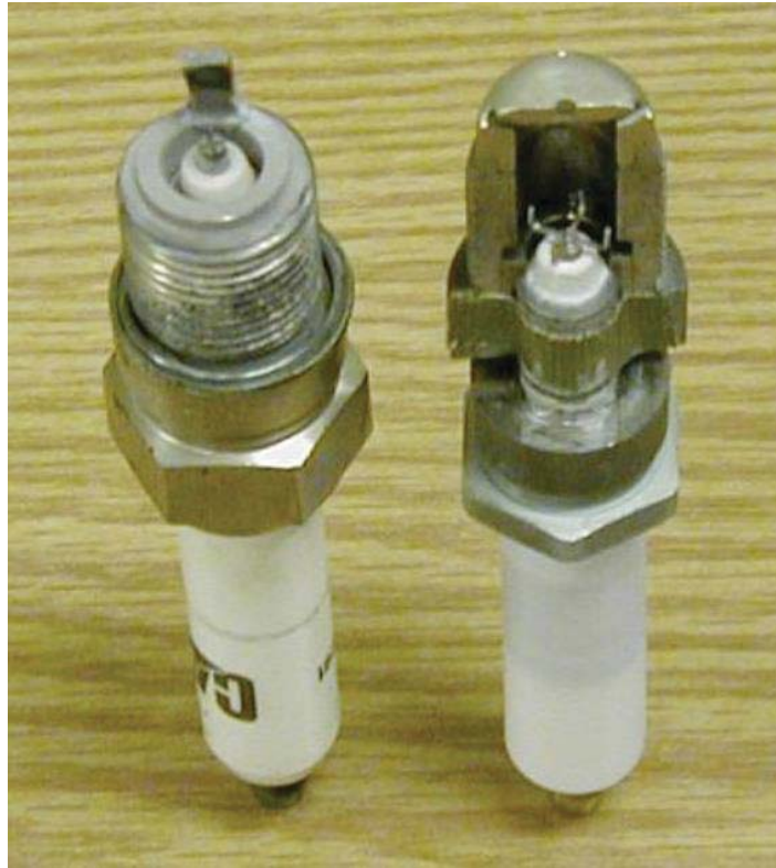
Figure 6: J-gap (left) versus prechamber (right) spark plugs.
