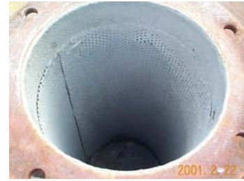
Figure 8: Inside of a muffler with Siloxane residue
