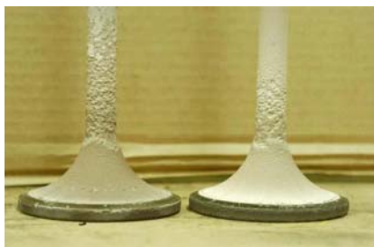
Figure 4: Exhaust valve with Siloxane buildup
