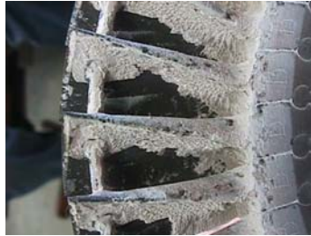
Figure 7: Siloxane build up on Turbocharger turbine wheel
