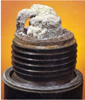
Figure 6: Spark plug contaminated with Siloxanes
